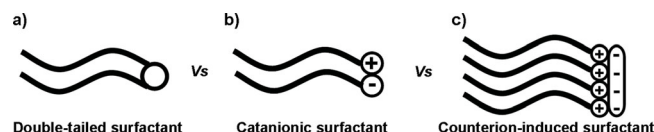
Figure 1. Comparison of three different methods to prepare vesicles: a) a method based on double-tailed surfactant; b) a method based on mixed cationic/anionic (called “catanionic”) surfactants; and, c) the counterion-induced surfactant method reported herein.
